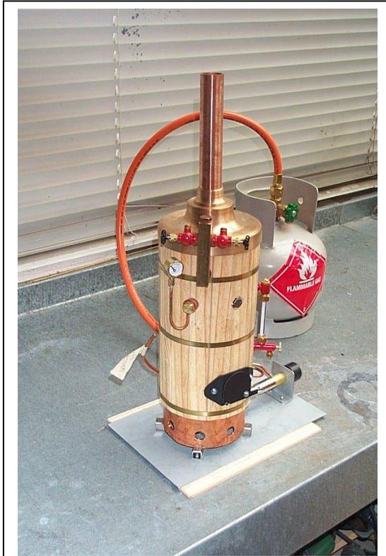
**LPG fired vertical boiler made for friend**
