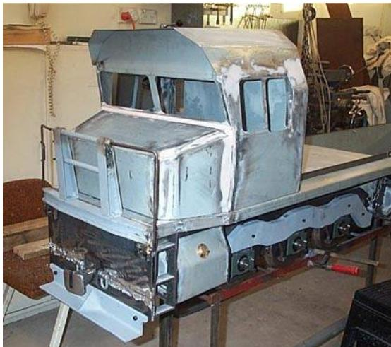
**Built up cab structure for the DXR.**
