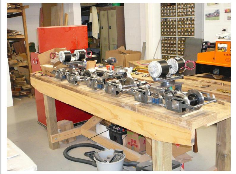
**The three bogies showing how motors are mounted**
