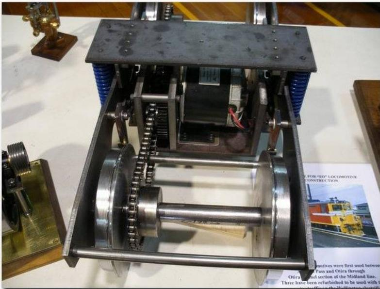
EO Bogie showing motor and drive train
