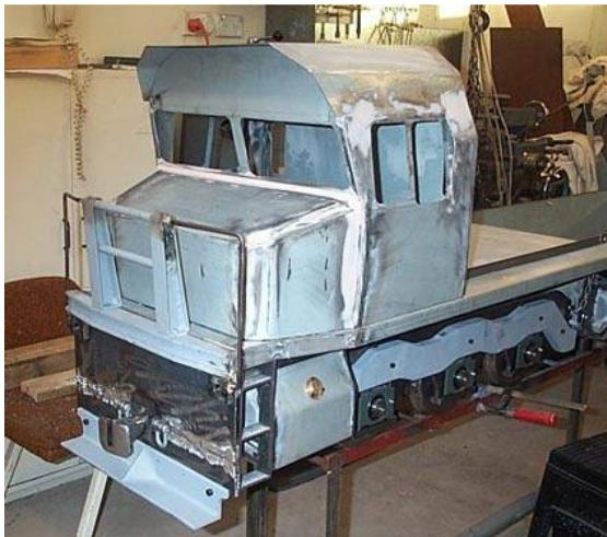
**Built up cab structure for the DXR.**
