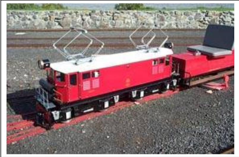
**EC9 in all it's splendour. Note the air tanks on the front and rear and how the bogies extend from under the body frame.**
