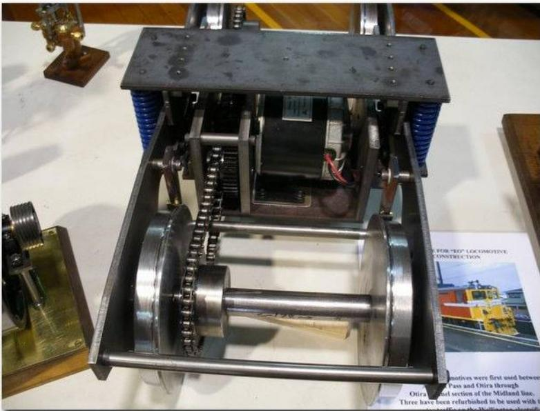
EO Bogie showing motor and drive train
