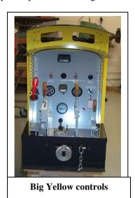
I fitted out the driving end with a gated control lever for which forward and reverse control is obtained, hand brake, train brake control, Hydrostatic Dump valve control and instrumentation. This loco is now in regular use at the track.
