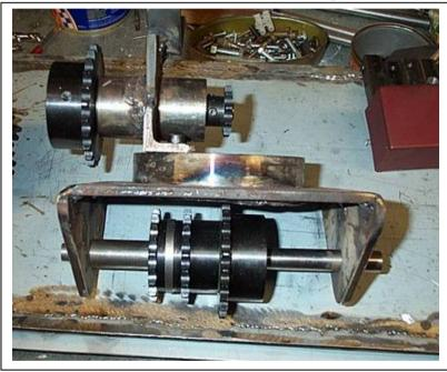
The chain drive goes through the trunion to the bogie below. Both axles are driven from the double sprocket on the left
