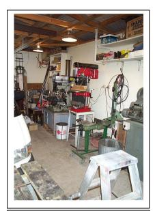
The workshop showing, welding corner, milling machine, drill press and saw
