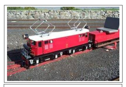
EC9 in all it's splendour. Note the air tanks on the front and rear and how the bogies extend from under the body frame.
