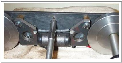
Hydraulic braking system with steel shoes and Holden wheel cylinder.
