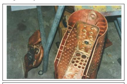
Copper boiler construction showing the shell and stays. The fire tubes can be seen at the end of the firebox.
