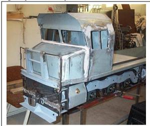
Built up cab structure for the DXR.
