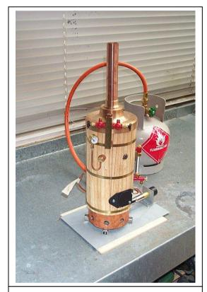
LPG fired vertical boiler made for friend
