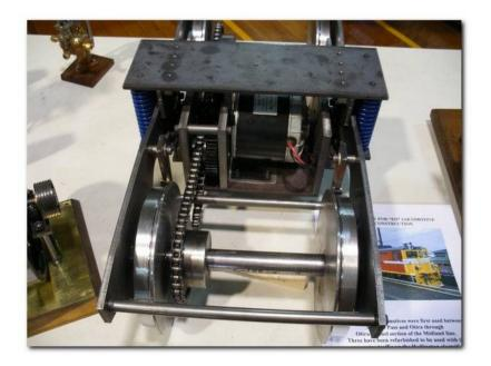
EO Bogie showing motor and drive train
