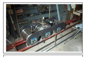
DXR Bogie Motor below trunion and Brake cylinder mounted at right hand end.
